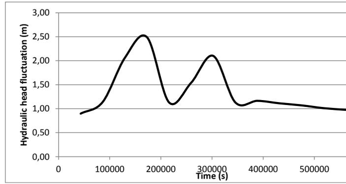
**Fig. 2 Variations of the hydraulic head measured at different distances to the riverbed after a flood and during recession**
