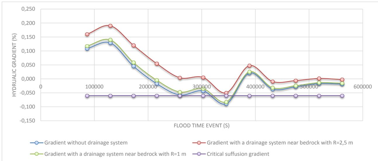
**Fig. 4– Drainage system positioned near surface of aquifer (9 m from the bedrock) with different radius. The red line describes the hydrograph of the fig.2 and 3.**
