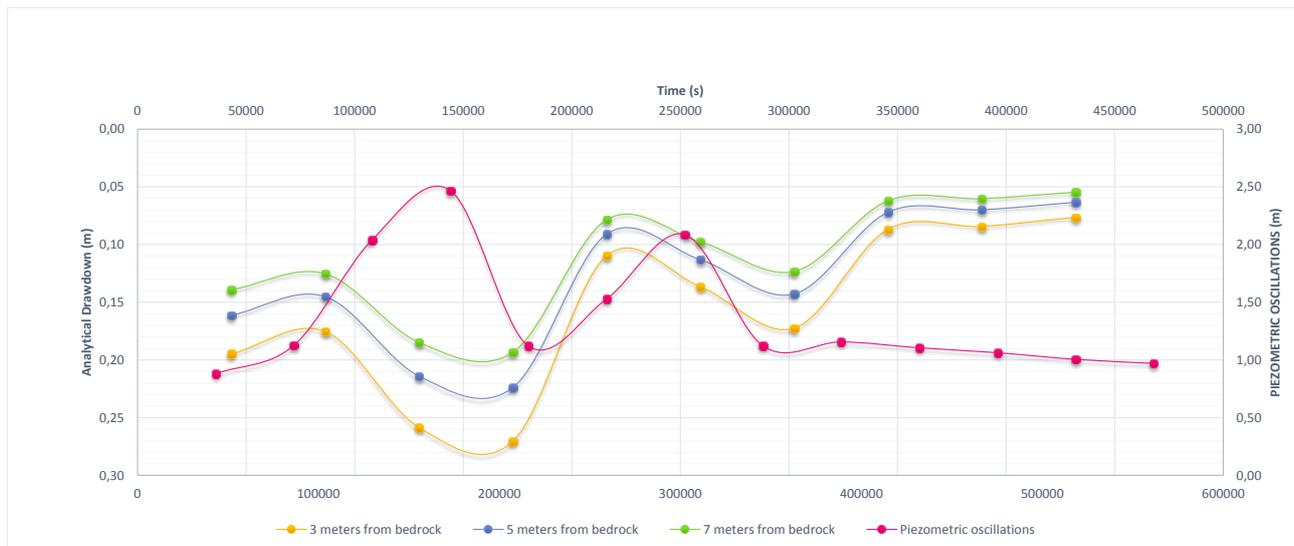
**Fig. 3 – Analytical drawdown 10 meter far from the river, with the drain arranged to different elevation with respect to the bedrock**
