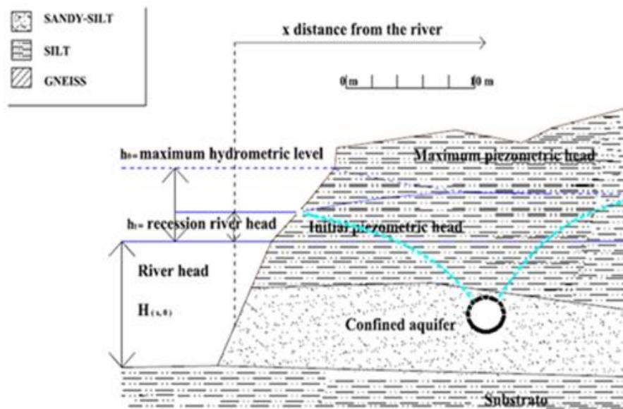
Fig. 1 –Cross section of the aquifer and of the watercourse
